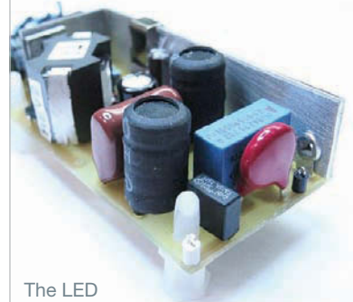
The LED driver detailed in DER-340 uses Power Integrations' LinkSwitch-PH power-conversion ICs.
